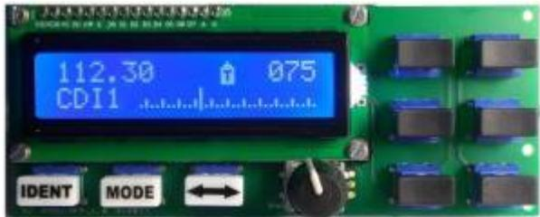
The Multi-Function Panel combines the six functions that are possible with the avionics module described above. Use the buttons on the side to switch between functions. The functions COM1, COM2, NAV1, NAV2, ADF and XPDR are available. I tried to synchronize the functions with the flight simulator, but these commands are often not supported by the developer of the aircraft panel.
