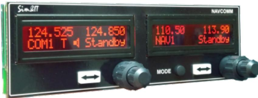
For the version with dual encoders, the inputs of the Arduino are only sufficient for connecting 4 buttons, which are then the two swap buttons, the mode button on the NAV and the push button on the rotary encoder. The audio functions TRANS, RECV, and IDENT are controlled via the [Audio-Panel](#). For this version I also used LC displays with a red background. These displays have a very limited lateral viewing area. The contrast decreases
