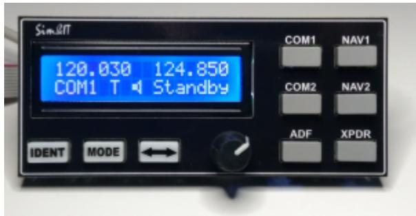
A black acrylic plate was laser-machined for the structure shown. Six 2.5 mm stud bolts were inserted into the plate to which the circuit boards are mounted.
