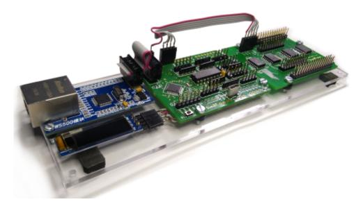
The figure shows the complete assembly of the controller with the port extension and the Ethernet module. With this extension it is possible to emulate switches of the panel of a small aircraft. This includes starter, light switch, fuel pump, tank, flaps, gear.
