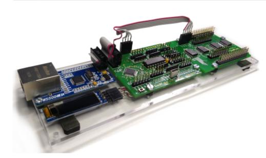
The figure shows the complete assembly of the controller with the port extension and the Ethernet module. Since the controller and the port expansion are in Arduino format, both boards could be mounted on top of each other with the appropriate distance if necessary.
