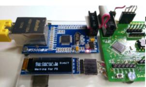
The display is an OLED display with a resolution of 128×32 pixels, which was connected via 4 lines as an I<sup>2</sup>C device. The display controller is a SSD1306. Because of the small size of the Arduino's memory a very simple library was integrated. This library is named **ss oled** in the Arduino IDE.
