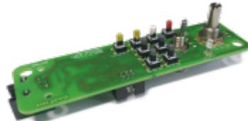
I have adapted the circuit based on the FREDI-1.8C of the [FremoDCC](#) with an SMD type of the ATmega328 and a different voltage regulator, as there were problems with the used LM2936. The [STEC11B03](#) was used as the rotary encoder, the slotted 6mm axis was shortened. Types with high light output (approx. 1000mcd) were used for the LEDs, so that the resistors were changed from 470R to 2.2k.
