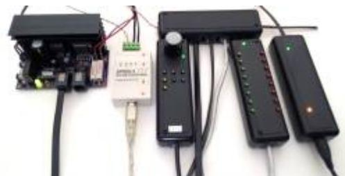
To enable speed controllers and other components to communicate with a PC as a control centre via LocoNet, an interface is required to buffer the signals from and to the PC and to implement communication with the LocoNet. The first draft of the **LocoBuffer** was created by [John Jabour](#). This page is only available via the [Web Archive](#).
