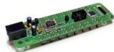
I have taken over the circuit and assembly of the connection side to the Loconet from the [LocoIO Keypad](#) and replaced the PIC with the ATmega328. I used the SMD type in the TQFP housing, as the DIL type should not be used for new designs according to the website. And so I was also able to use the circuit design of my flight simulation devices.
